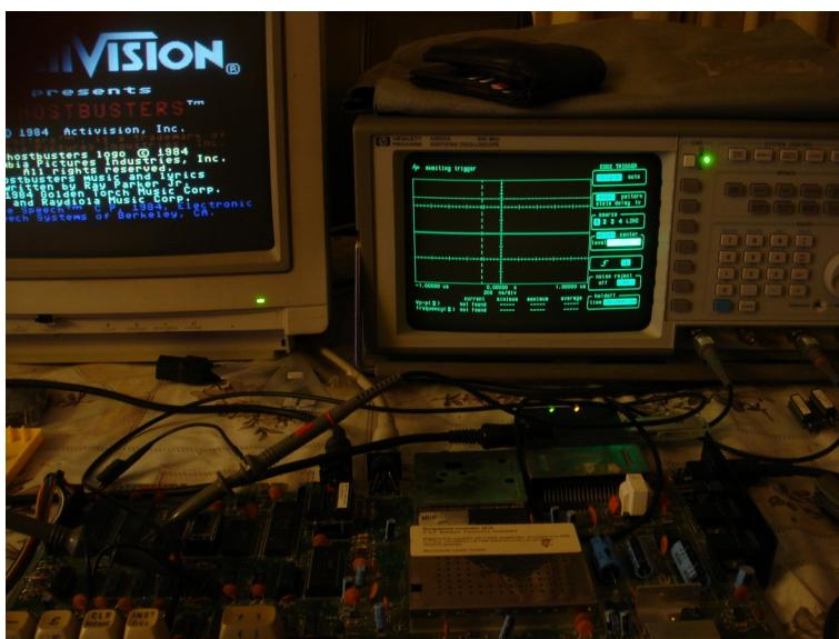
The trigger level of the oscilloscope is set to 3.75V and it keeps waiting indefinitely for a trigger. Only when increasing to 4V it does trigger, but then just shows the stable high logic level:
