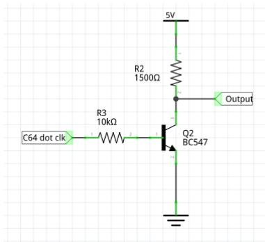
The idea is good, but it doesn't work. I have built the above circuit and it results in a flat voltage at the output:
