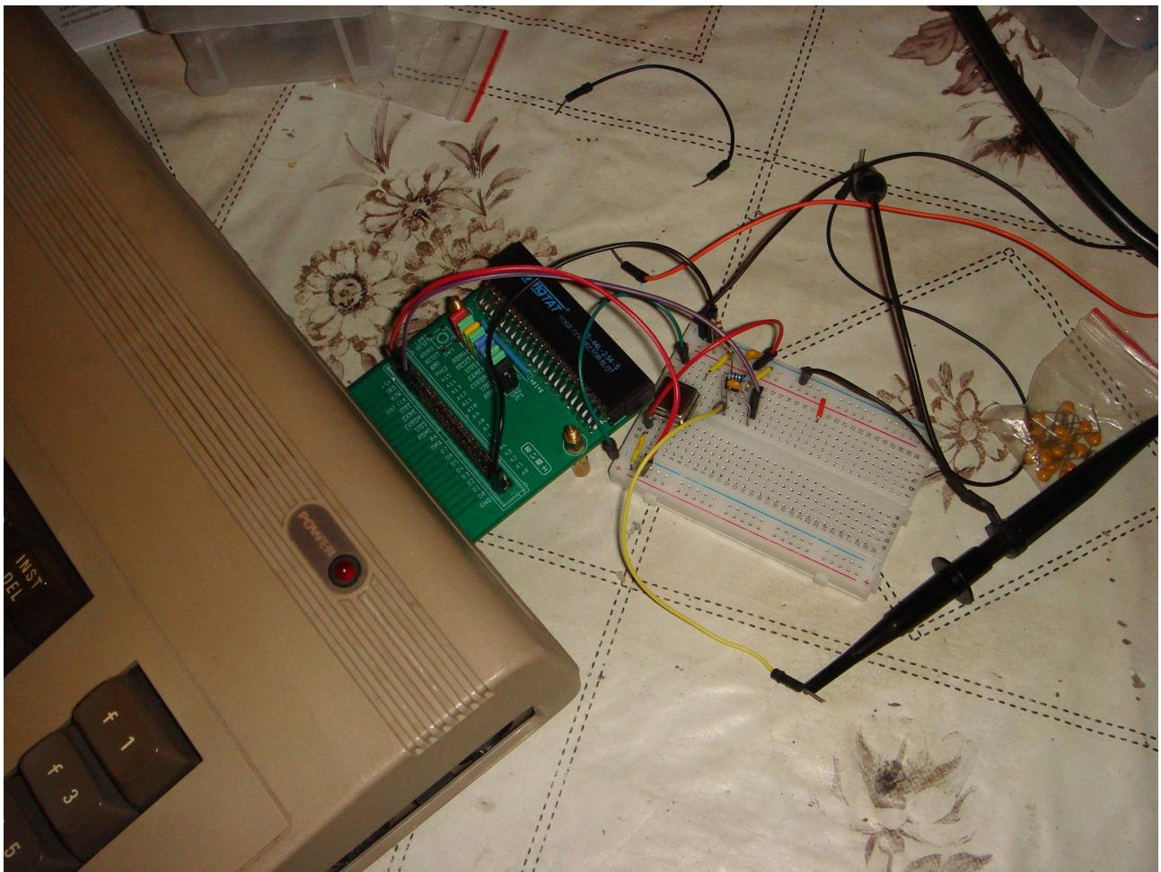
Why doesn't dumping the clock into a BC547 work? The answer is the Miller effect. If there is a capacitor between the input and output of an inverting amplifier, the amplifier will not just amplify the signal, but also the capacity of the capacitor, the capacitor will appear to be much larger than it really is:
