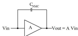
Why is this? Well suppose you amplify the voltage by a factor 2. Then the voltage difference between input and output is also two times as high. With a two times higher voltage you can store twice as much energy in the capacitor, so on the input side, it will appear to be twice as large.
