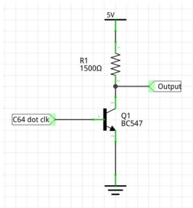
I haven't tested this: While Amstrad might have been okay to dump a clock signal into the base of a transistor, this won't work on a Commodore 64, since it will drop the dot clock to ground. The dot clock is primarily used by the VIC-II, so building the above circuit would crash the Commodore 64. Further, although I believe it ain't harmful (NMOS pull-up is weak), there is no proof the Commodore 64's clock chip is able to handle the higher currents that will flow.
