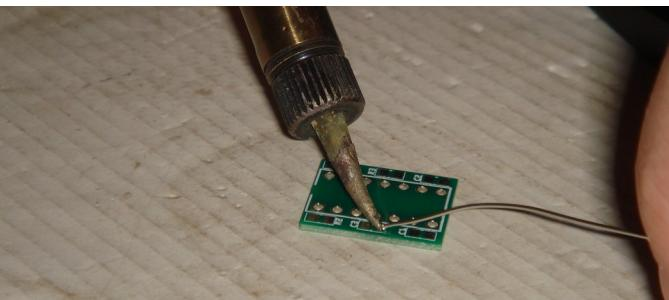
Pickup a component with tweezers. Hold your soldering iron in your other hand. Heat up the pad you just applied
