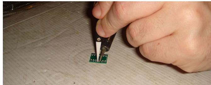
Remove the soldering iron and the component will fix into position. Now, apply solder to the other side of the component:
