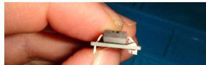
Plug the included headers into an IC socket. You can also use a breadboard:
