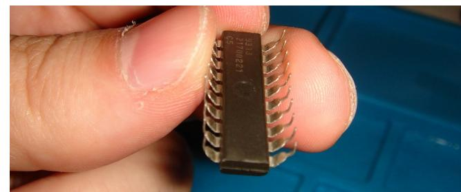
**Warning:** Unlike on the photo's, the included label should not yet be attached to the IC, because heat from the soldering iron will make it turn brown. Attach the label after soldering is finished.
