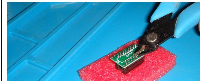
Place the IC onto the PCB and solder it into place:
