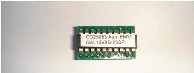
The EMMU is plug and plug and functions like the original EMMU. It can be plugged into the mainboard. There is no need to install U35 and therefore the replacement is compatible with mainboards that don't have position U35.
