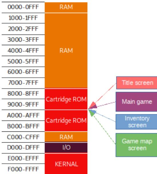
As parallel ROM on the Super Guppy cartridge works like a traditional bank switched cartridge, the Super Guppy is suitable for the overlay memory model and its KERNAL replacement feature comes in handy.
