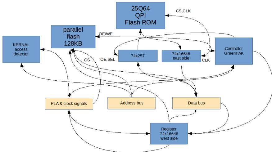
A schematic diagram of the Super Guppy Cartridge
