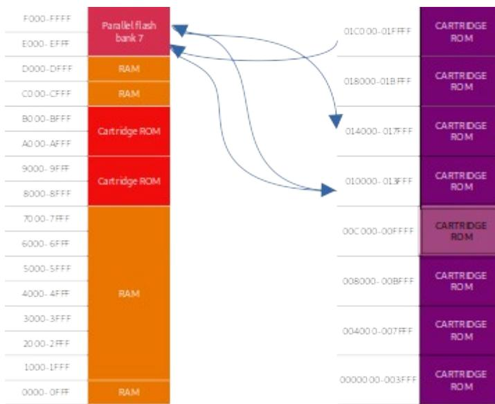
In an all-code-outside memory model, code can freely jump from anywhere to anywhere in parallel flash memory. If code needs to call a routine in another bank, it can call a far-call wrapper in the bank 7 ROM that is mapped into the KERNAL memory space.
