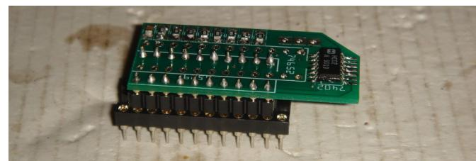
Next, solder the socket and add the 74xx65x, but, if you are replacing the keyboard SPI of the Plus/4, do not solder the socket, but solder the 74xx65x directly!
