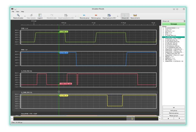
The WE pulse ends about 50ns before end-of-cycle. At that time the data bus is fully stable, and doing it this avoids a race at the end of the clock cycle to end the write pulse before the address bus starts to change (as is the case with EasyFlash). There is all the time in the world, and this will make the cartridge a lot less senstive to SRAM speed and the speed of other components than the EasyFlash cartridge is.
